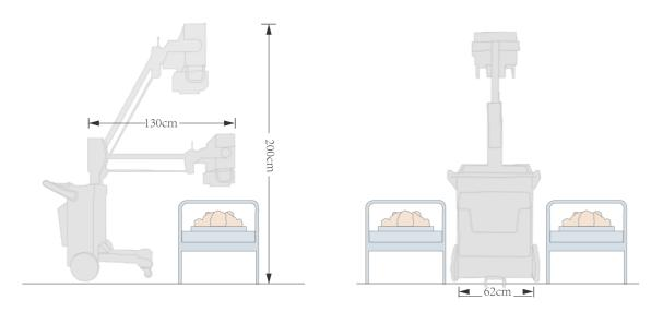
• PLX5100 uses lightweight materials, the weight of the whole machine is less than 150KG, innovative mechanical design, light and flexible to move; dislocation brake system, safe and reliable braking.
